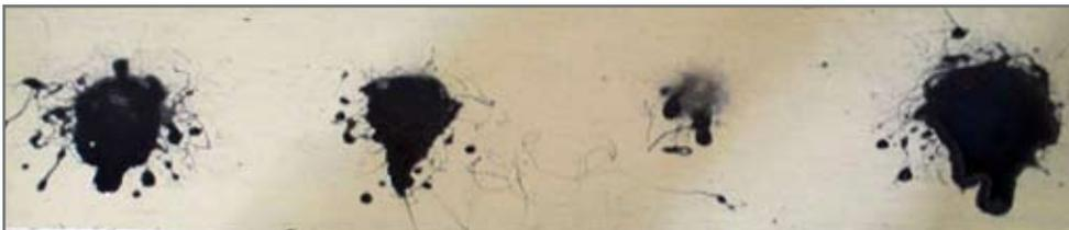
Spray pattern using a commercial grade lubricant.
